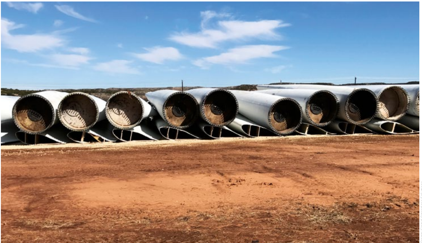
Traditional wind turbine blades cannot be recycled and often end up in landfill, however some companies are looking at options to develop recyclable blade, or at ways to reuse them.
