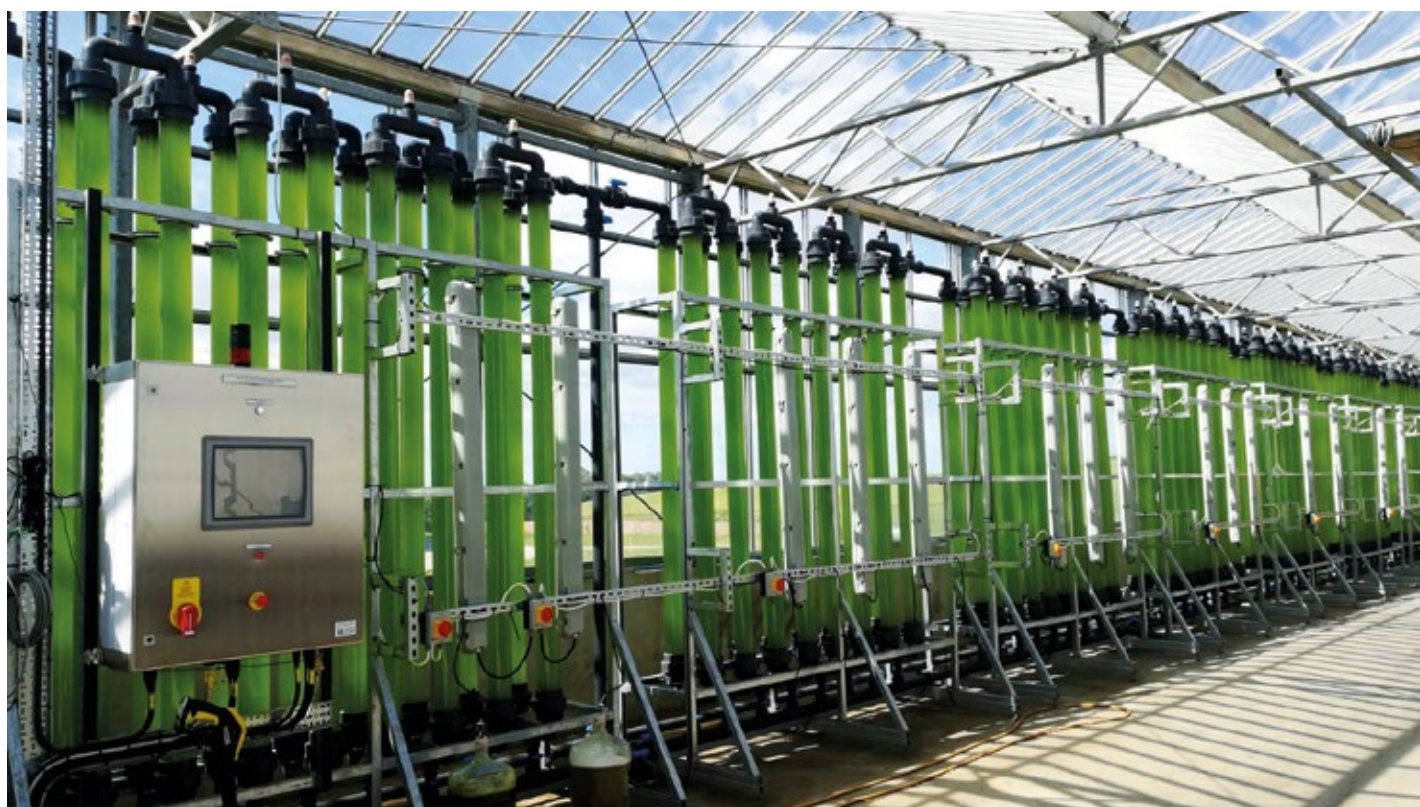
A team of researchers at Swansea University are using food and farm waste to cultivate microalgae as part of the Interreg North-West Europe project ALG-AD 26 .
