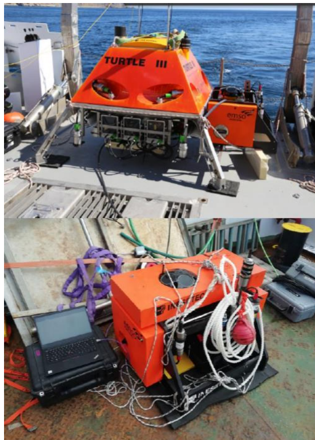
Figure 12– EGIM sensor module (top: attached to TURTLE, bottom: standalone)
