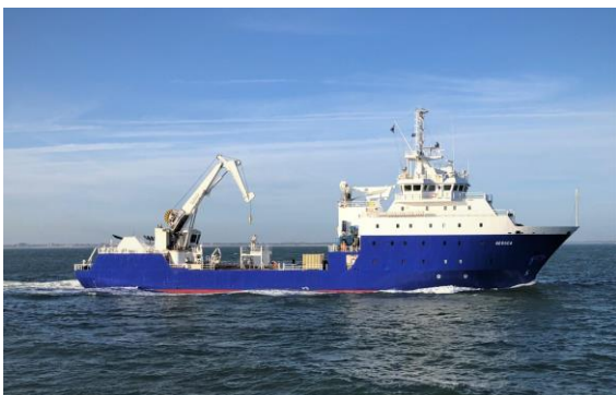
Fig. 5. Example of suitable multi-purpose work vessel for O&M in the wave energy farm (From: [25]).
